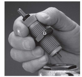
Screw the sizer die into the reloading press.
