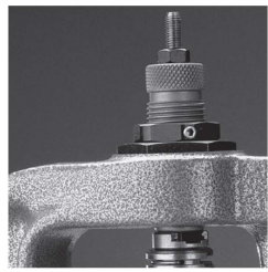
Notice the sizer die adjusted so it contacts the shell holder.
