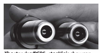
The standard RCBS steel dies shown on the left. The carbide sizer is visible in the carbide sizer die on the right.
