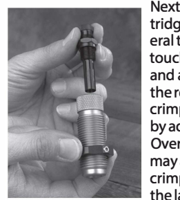
Seater dies in our 3-diesets use a "through-the-top" style seater plug as shown above. This allows for easy cleaning.
