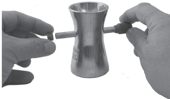
Photo 3 Insert tube and install retaining ring
