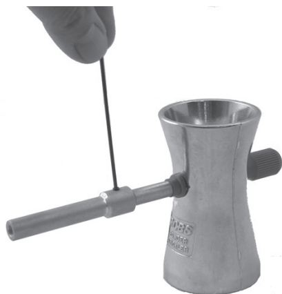
Photo 4 Secure extension tube set screw
