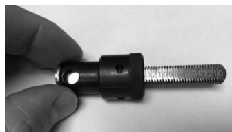
Metering Screw properly aligned
