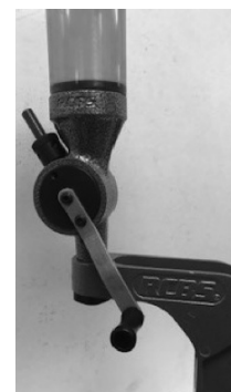
Dispensing Metered Charge (Handle Down)
