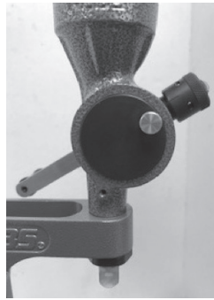
Cylinder position when setting for lightest load
