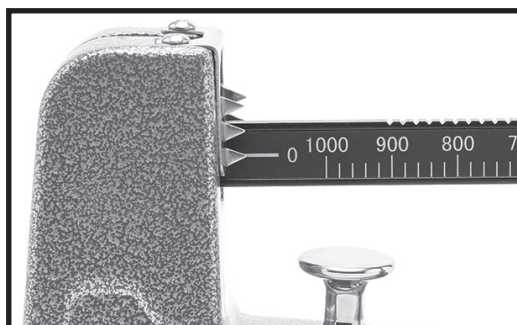
Photo 23: Bottom pointer at 0.5 grains below reference target load
