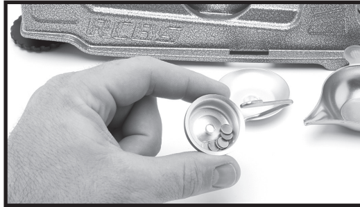
Photo 11: Weight holder containing non-magnetic material
