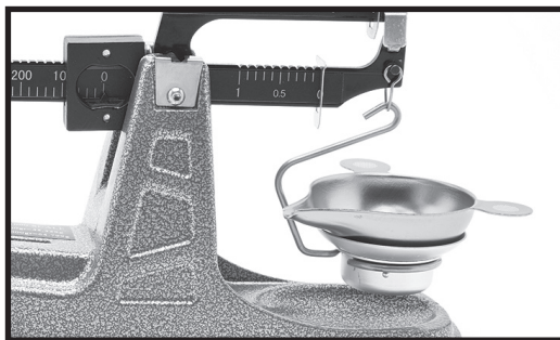
Photo 5: Place pan onto pan support
