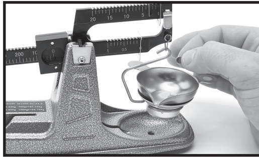
Photo 14: Add or remove calibration weights
