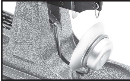
Photo 25: Scale pan placed into slot in base
