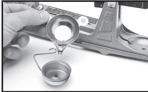
Photo 15: Place calibration material back into weight holder
