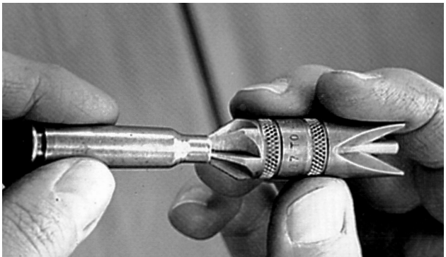
Lightly chamfer the case mouth to remove rough edges for easier bullet seating.
