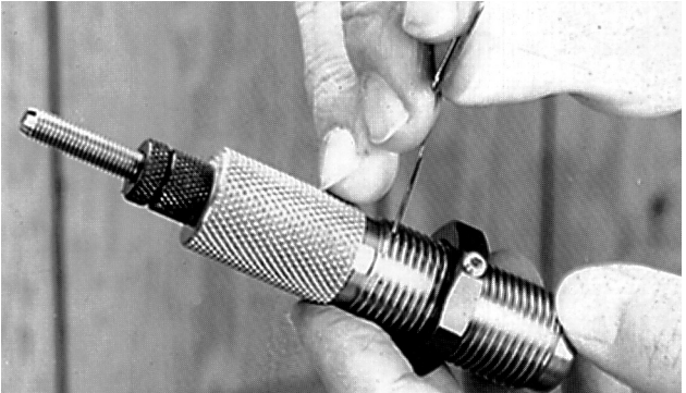
The vent hole, found on some dies, must be cleaned out prior to using the die.
