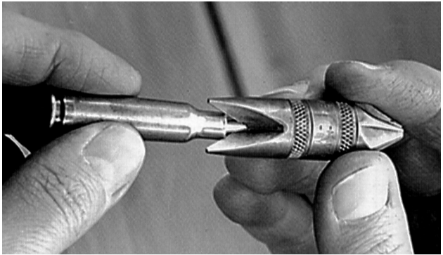
Use this end of the deburring tool to deburr the outside of a trimmed case.
