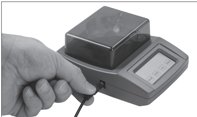
Photo 2: 9 VDC Power Supply
