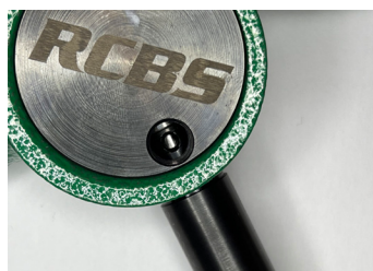
Correct Alignment for the Lock Screw
