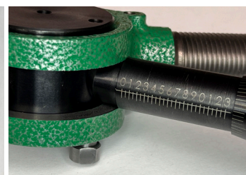
Correct Alignment of the Graduation Marks
