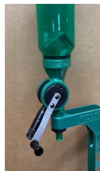
Filling Metering Cylinder (Handle Down)
