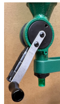
Powder Measure with Drop Tube installed
