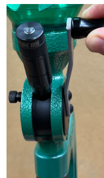
Dispensing Metered Charge (Handle Down)
