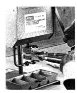
Fill the dipper aprox. 3/4 full of alloy. Tip the mould on its side.
