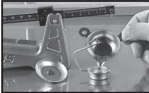
Photo 15: Place calibration material back into weight holder
