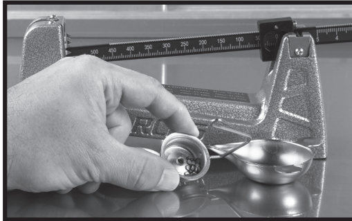
Photo 11: Weight holder containing non-magnetic material
