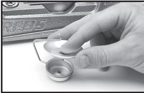
Photo 16: Secure pan support to weight holder
