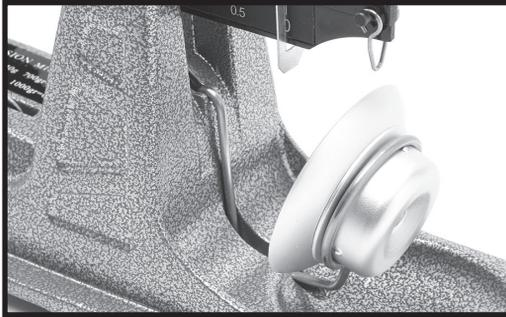
Photo 25: Scale pan placed into slot in base
