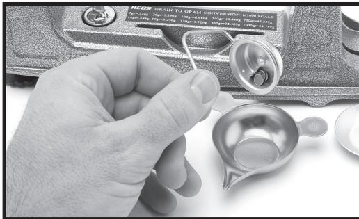
Photo 12: Place calibration weights into scale pan
