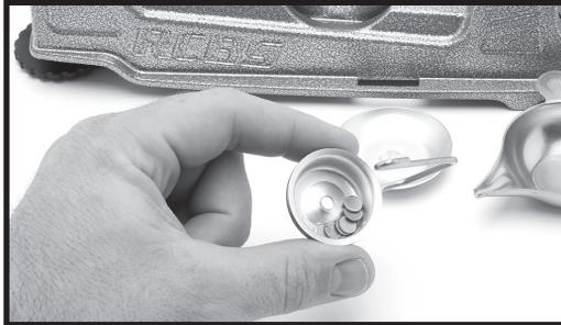
Photo 11: Weight holder containing non-magnetic material
