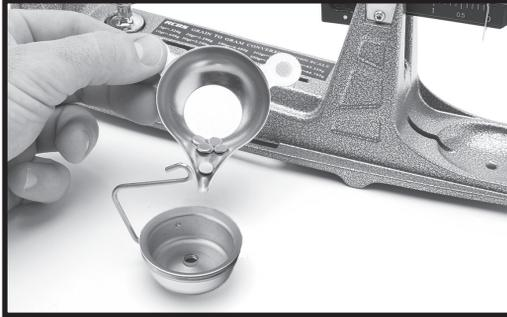
Photo 15: Place calibration material back into weight holder
