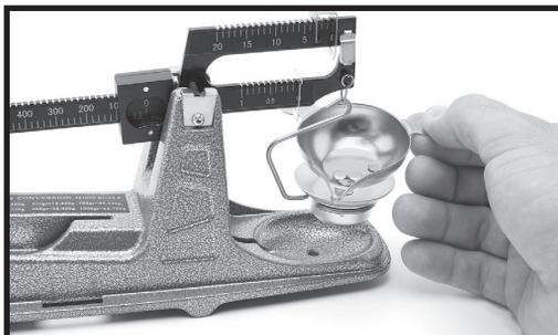
Photo 13: Place scale pan onto pan support
