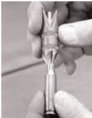
Lightly chamfer the case mouth with an RCBS Deburring Tool.
