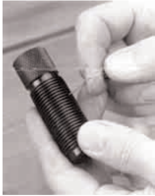
Use a straightened paper clip to clean the vent hole.
