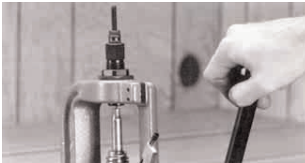
Adjust the sizer die in the press to properly size the case.
