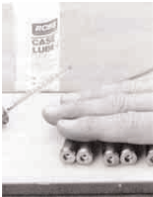
Roll cases on an RCBS Case Lube Pad for proper lubrication.
