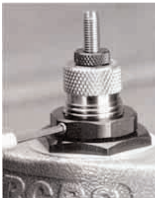
After adjusting the die, tighten this setscrew to hold the proper setting.
