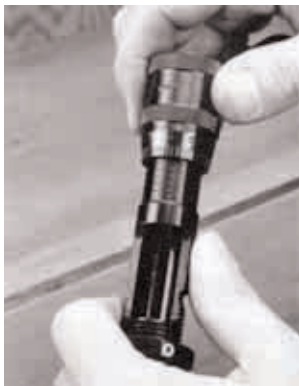
Each graduation on the seater die is .001".
