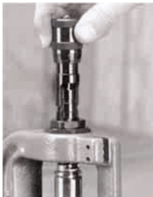
Turn the thimble clockwise to adjust the seating depth.
