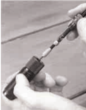
Before cleaning the vent hole, unscrew the expander-decap assembly from the die.
