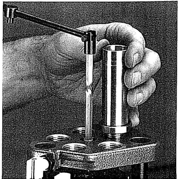
Photo #45: Install the powder measure adaptor into the top plate.
