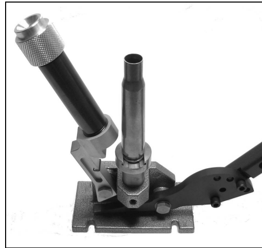
Pushing the handle down will move the primer feed arm into position.
