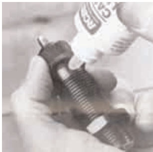
Fill the Lube Die with RCBS Case Lube-2.
